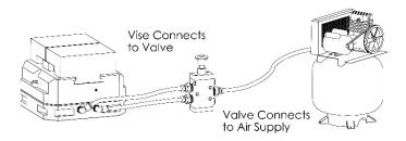
The switch box provides you the capability to operate the vise in a manual mode. Ensure it is set in your desired configuration.
