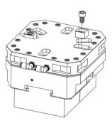
The included T-Slot nuts and vise keys will assist you in ensuring accurate alignment and security on the table. Install the vise keys to your desired configuration and align the vise with the table. Fit the T-Slot nuts into the table slots, align with
